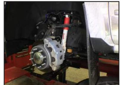
**STEP 5:** Loosen, then remove the two front Upper Shock Mounting Nuts on both sides of vehicle.
