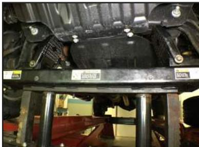
**STEP 4:** Remove front tires/wheels, and locate Upper Shock Mounts.
