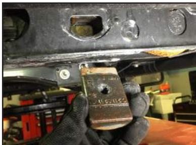
**STEP 12:** Use an air hammer to slide the Torsion Bar forward to clear the Torsion Key.
