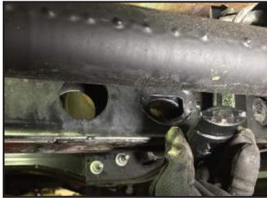
**STEP 16:** Install new Forged 3" 12.9 Adjuster Bolt make sure it has full thread engagement before removing tool.
