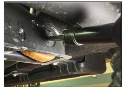
**STEP 13:** Remove OEM Torsion Key. Install ProRyde Torsion Key and slide Torsion Bar back into Torsion Key.
