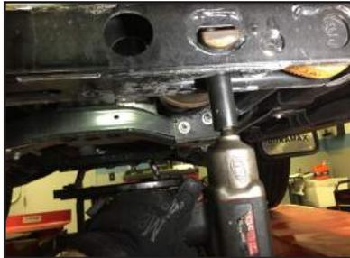
**STEP 10:** Using a tool specific to GM vehicles such as 88-8000 or similar, compress the key until it clears the Threaded Adjuster Bracket.
