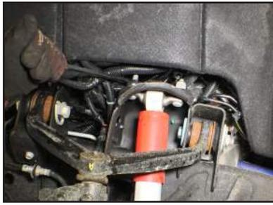
**STEP 6:** Install new front Shock Extender Spacers. Compress top of each shock downward to access the two threaded shock mount studs, and install one Shock Extender Spacer on each of the four studs.
