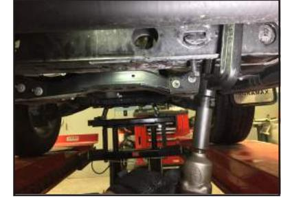
**STEP 11:** Remove OEM Adjuster Brackets and 88-8000 tool.
