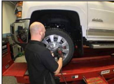
**STEP 20:** Lower the vehicle, jounce suspension and measure ride height of EACH SIDE of the vehicle. Measure from the bottom of the wheel/rim to the lip of the fender.
