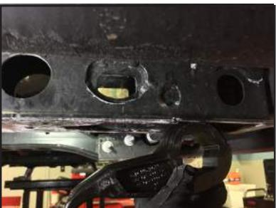
**STEP 14:** Use a Torsion Bar Unloading/Loading tool to compress the key until it clears the Adjuster Bracket slot.
