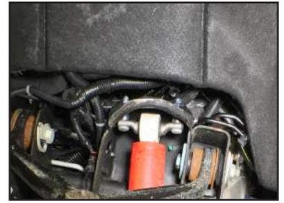
**STEP 7:** Reinstall shock and secure using four new Low Profile Shock Mount Nuts supplied with this kit.
