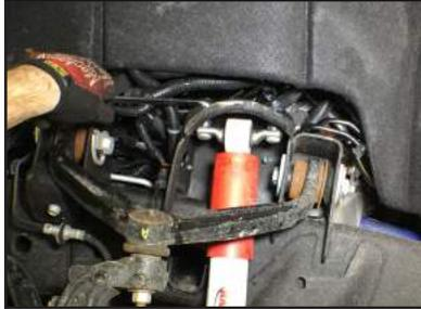
**STEP 8:** Locate the OEM Torsion Key. They are located where the torsion bars are received into the Crossmember between the frame.
