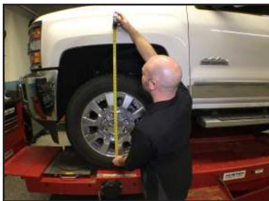
**STEP 2:** Position vehicle on a stable, flat surface or automotive lift. Chock wheels. Be sure engine is turned OFF and vehicle is in PARK.
