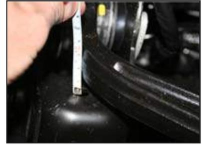
The gap between the Upper Control Arm and Bump Stop should be 1/4" to 1/2" with weight on the wheels.
