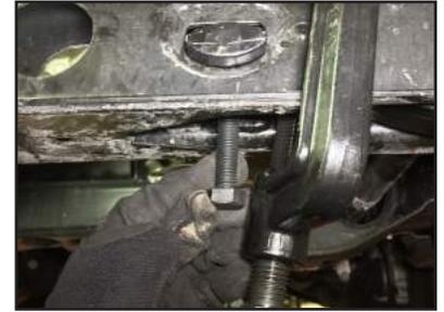
**STEP 17:** SLOWLY release tension on the Unloading Tool until it can be fully removed, then repeat Steps 12 through 16 on other side of vehicle.
