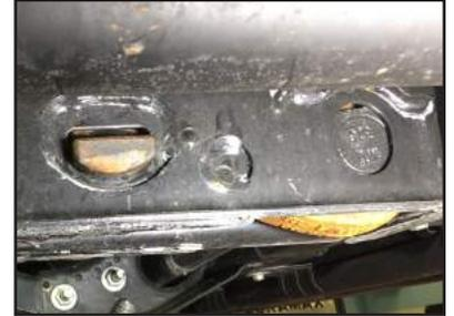
**STEP 9:** Using a 22MM socket, loosen and remove the OEM Torsion Key Adjusting Bolt.
